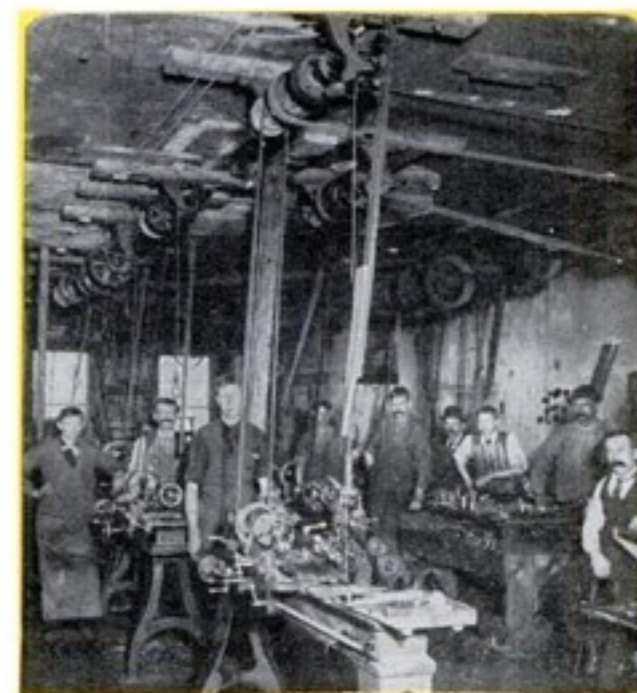
Machine-tool shop of 50 years ago presented maze of overhead pulleys.
