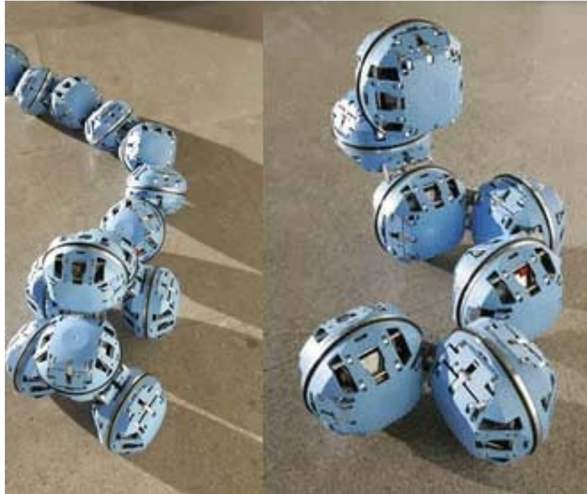
Figure 2-7: ATRON system, consisting of hemispheres connected by a rotary joint, and connected to each other by a right-angle bracket. The hemispheres are 110 mm in diameter. (Østergaard [71])
