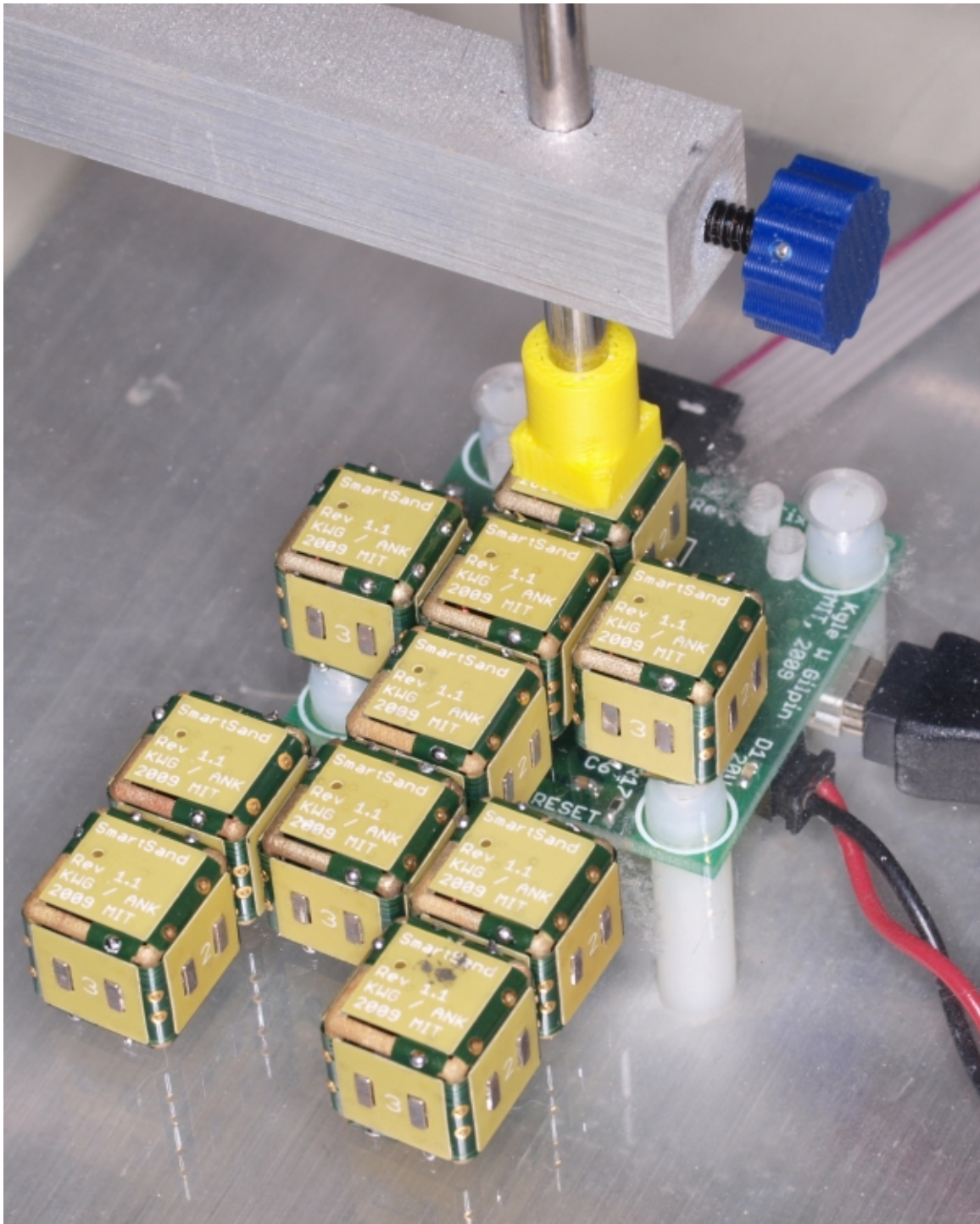
Figure 4-11: Experimental apparatus showing a humanoid after a completed disassembly trial. The clamp holds the root module in place onto a bed of pogo pins, which provide the root with power and a data connection to the PC.
