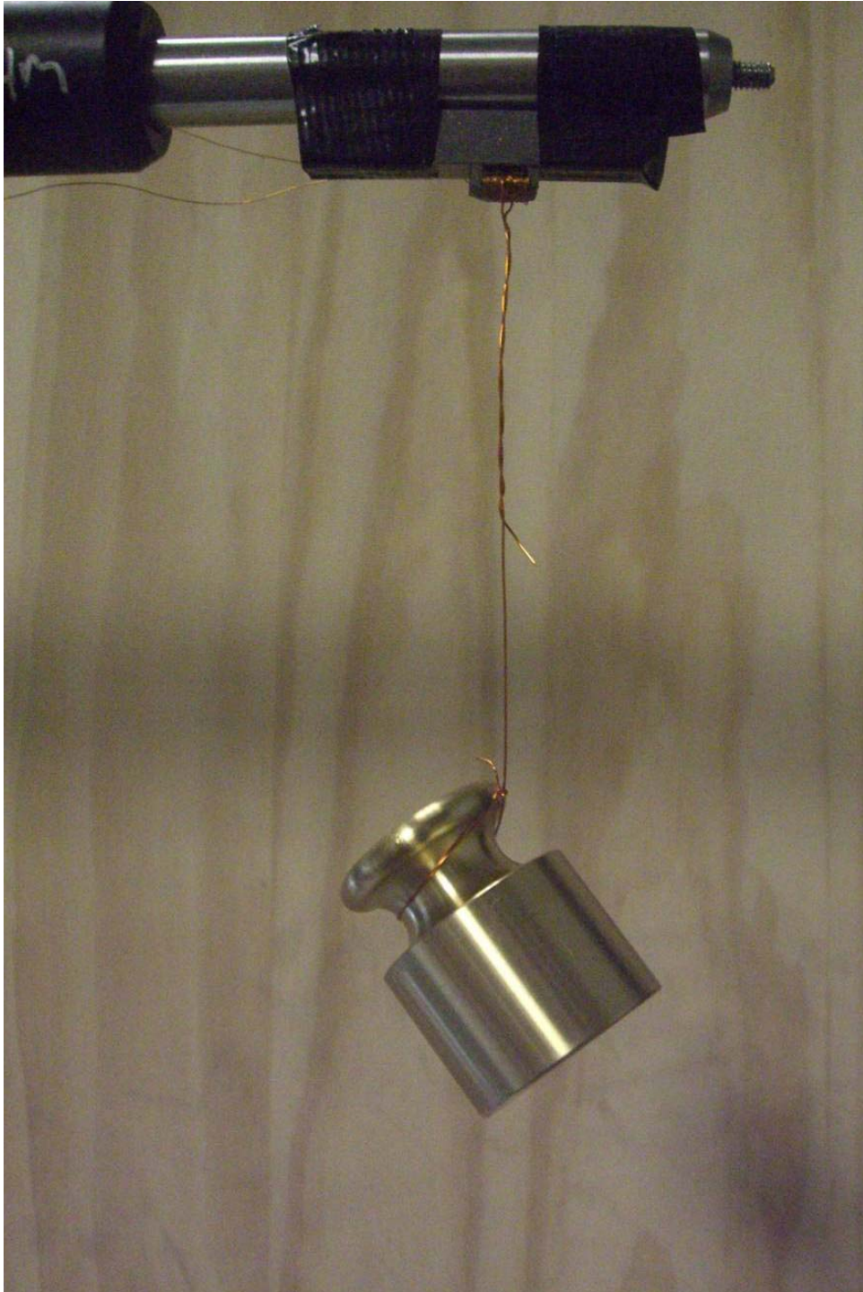
Figure 3-10: Electropermanent magnet, switched on, holding up a 250g test mass.
