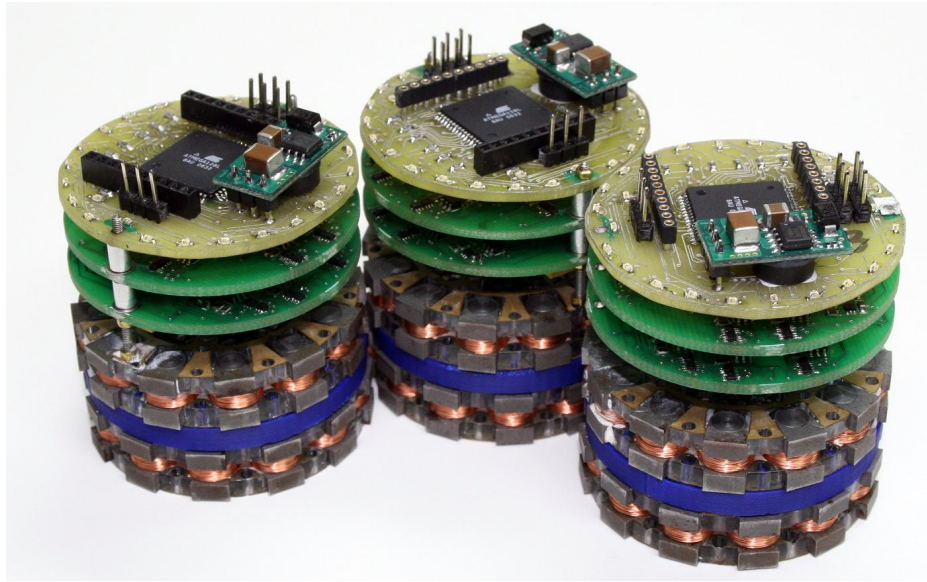
Figure 2-9: The planar magnetic Catoms. The cylindrical modules are 45 mm in diameter. They use an array of electromagnets for cooperative actuation and inductive power transfer and communicate using an array of infrared LED's. (Kirby [54])
